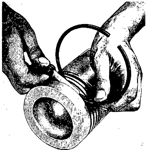
Check the axial play of the piston rings
