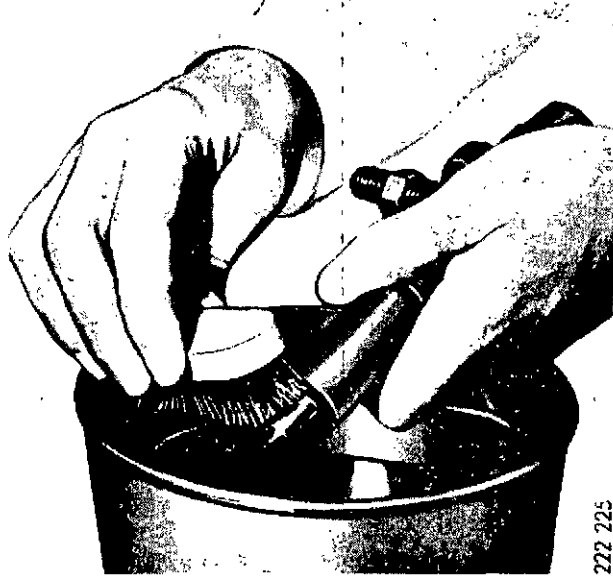
Clean the outside of the injector
