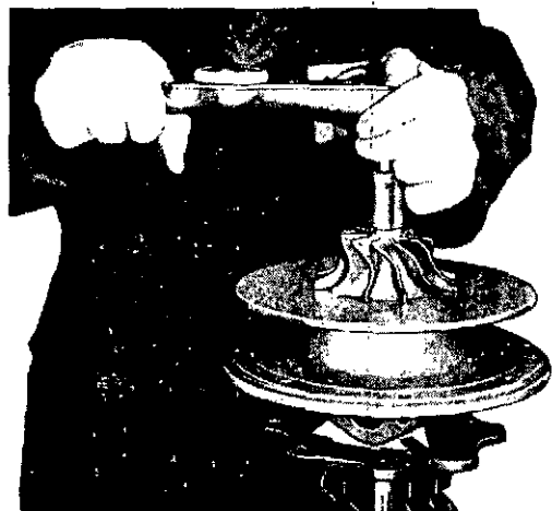
Tighten the locknut
