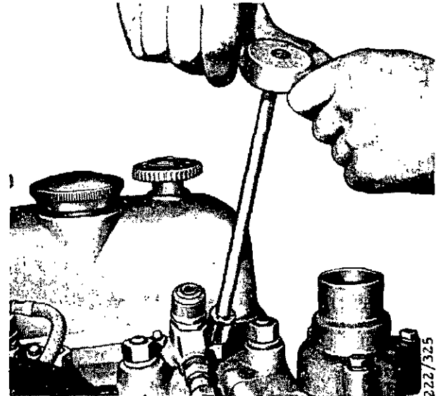
Always use a torque wrench in tightening the injectors
