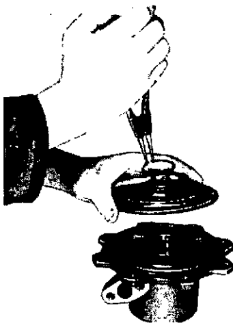
Fit the support plate and the lock ring
