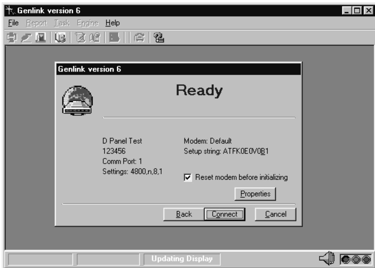
Figure 5 — Dial Up the Remote Generator
