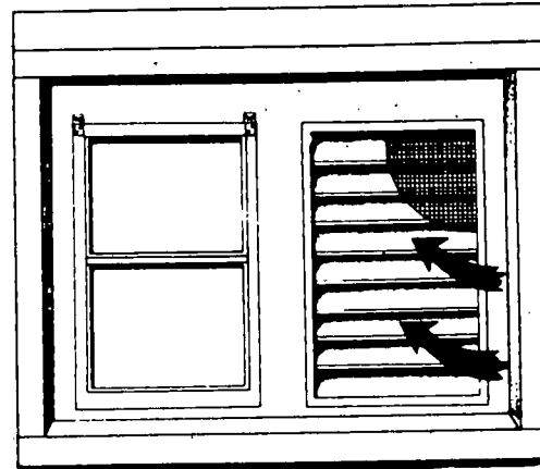
Figure 12. Air Opening with Fixed Louvers
