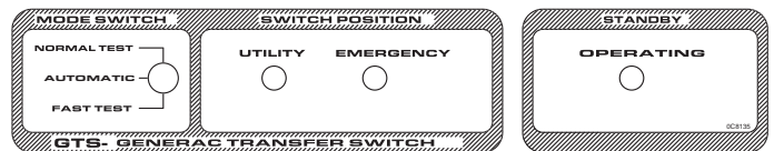
Figure 3.6 — System Test Switch, Standby Operating LED, and Switch Position LED
