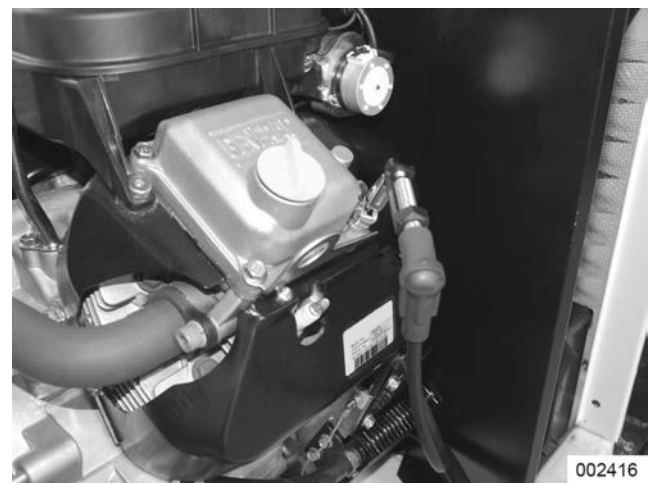
Figure 4-34. Checking Ignition Spark
