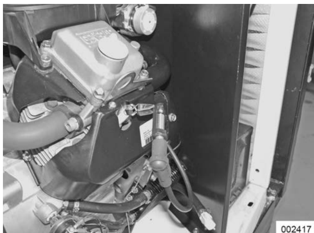
Figure 4-35. Checking Engine Miss
