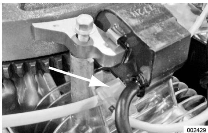
Figure 4-46. Cylinder Two Shutdown Wire
