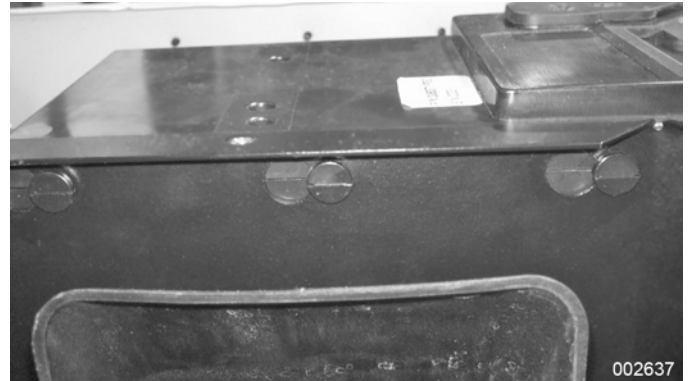
Figure 6-3. Tabs on Controller
