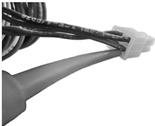
002450 Figure 1-2. Back-Probing Molex Connector
