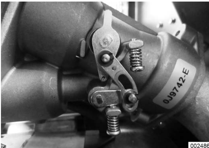
Figure 2-16. Stepper Motor Closed – Closes Both Venturis
