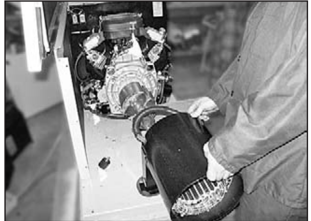
Figure 5. Removing the Stator
