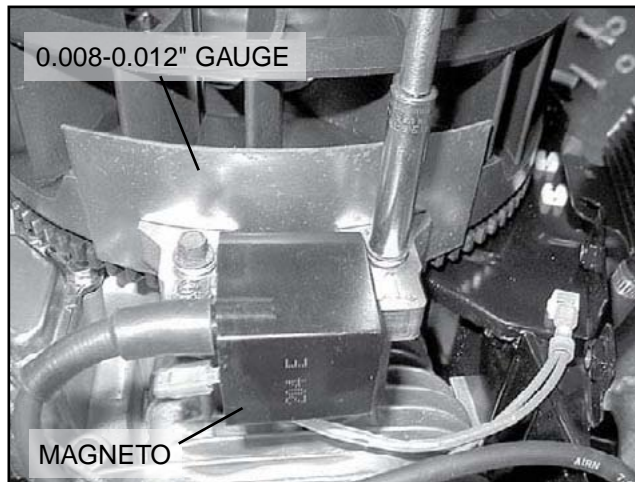
Figure 34. Setting Ignition Magneto (Armature) Air Gap
