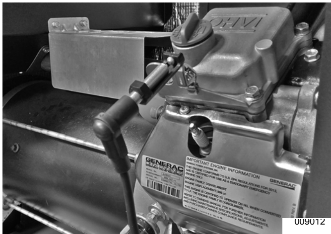
Figure 3-62. Checking Ignition Spark
