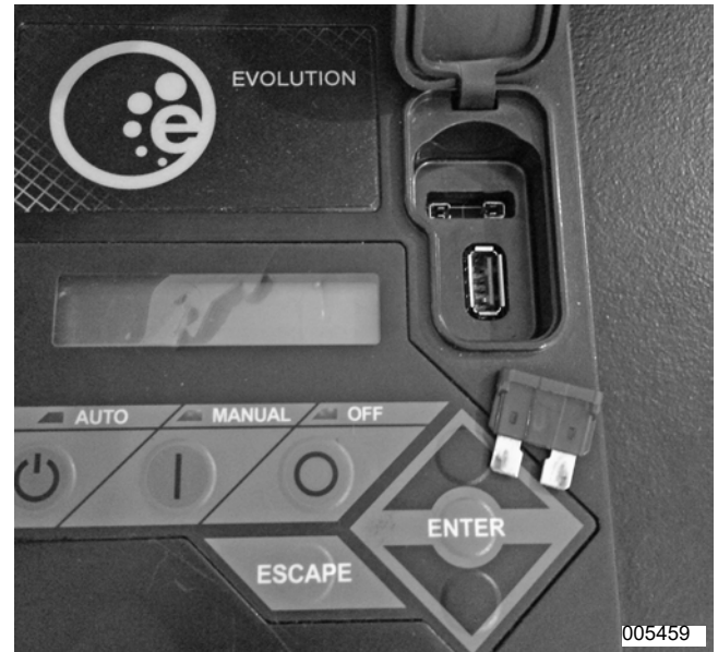
Figure 4-38. Remove 7.5 Amp Fuse
