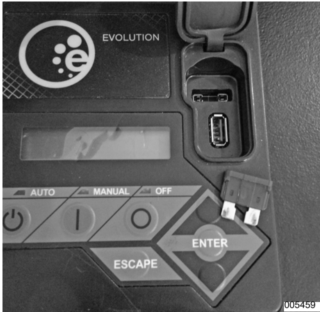
Figure 4-1. Remove 7.5 Amp Fuse
