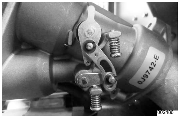
Figure 3-59. Stepper Motor Closed – Closes Both Venturis
