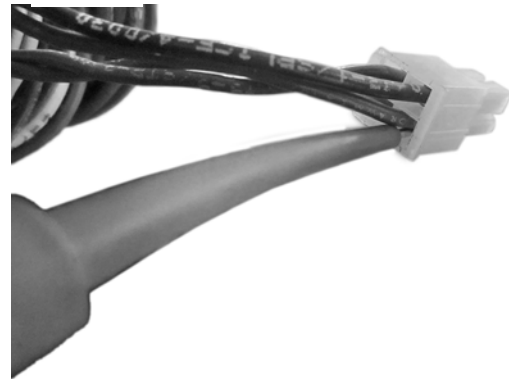
Figure A-2. Back-Probing Molex Connector
