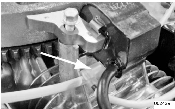
Figure 3-75. Cylinder Two Shutdown Wire
