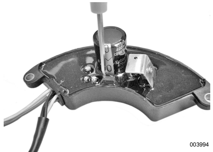
Figure 2-7. Voltage Regulator Adjustment Screw
