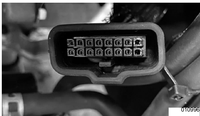
Figure 3-24. 16-Pin Harness Connector (CONN1)
