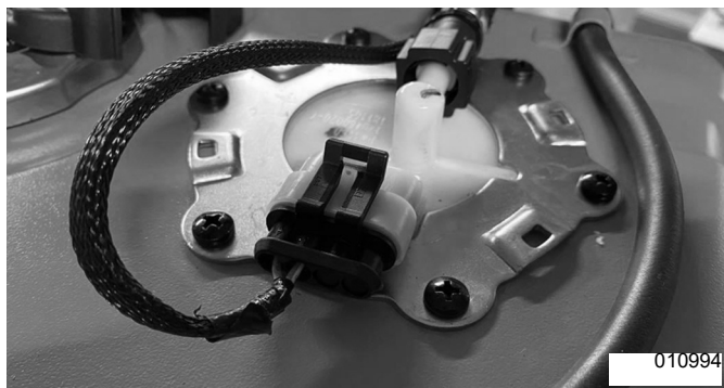
Figure 3-20. Fuel Pump Connector
