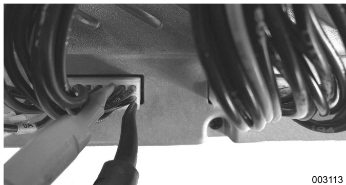
Figure 3-126. Back Probes in Use
