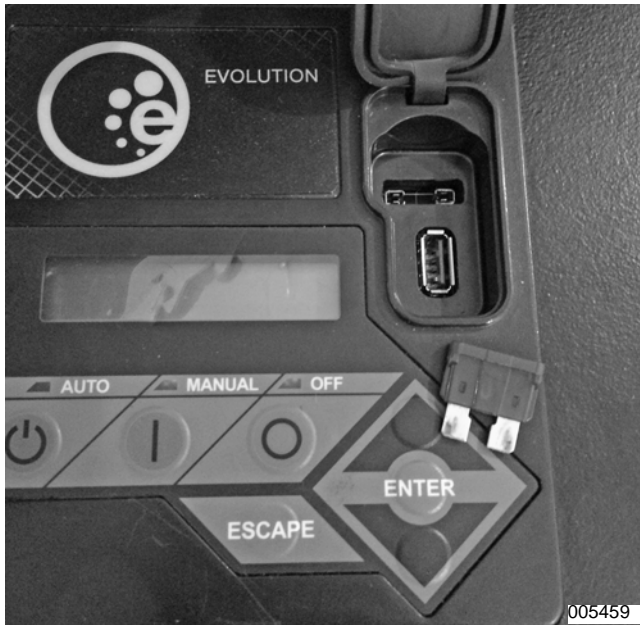
Figure 5-2. Remove 7.5 Amp Fuse (Evolution)
