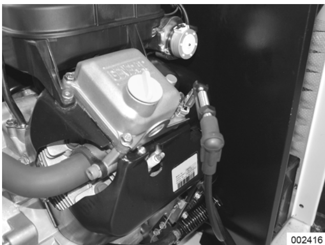
Figure 4-77. Checking Ignition Spark
