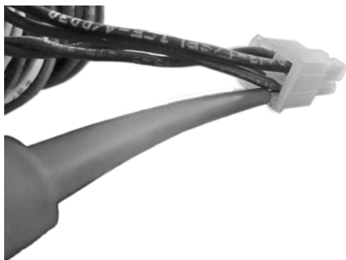
Figure A-2. Back-Probing Molex Connector
