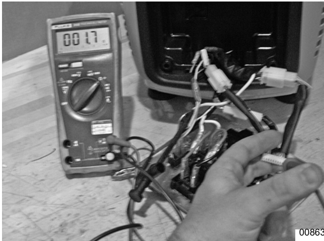
Figure 1-41. Test Ignition Coil
