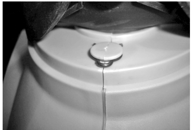
Figure 1-55. Remove Retaining Clip
