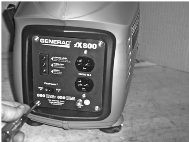
Figure 1-56. Remove Control Panel
