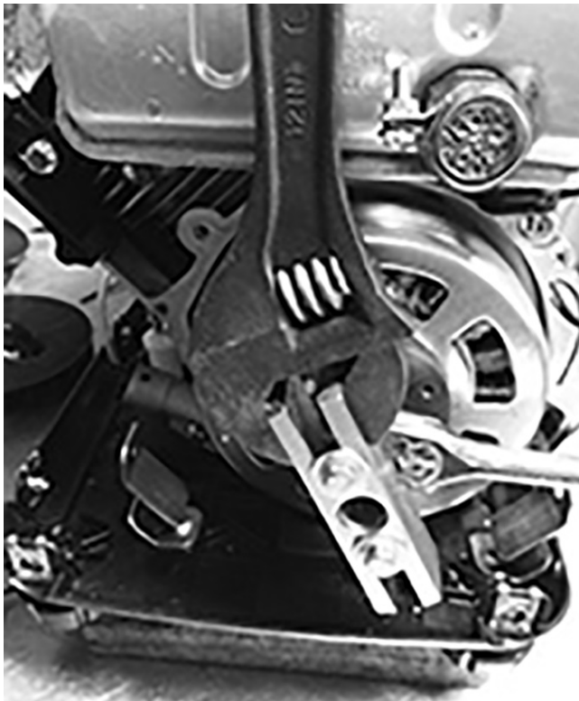
Figure 1-95. Breaking Nut Loose
