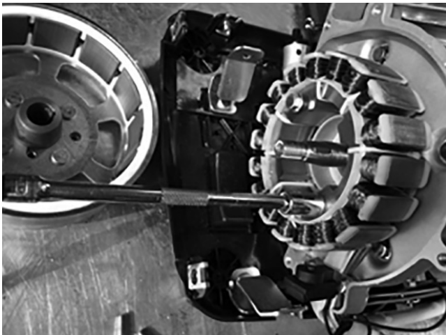
Figure 1-99. Remove Stator Assembly
