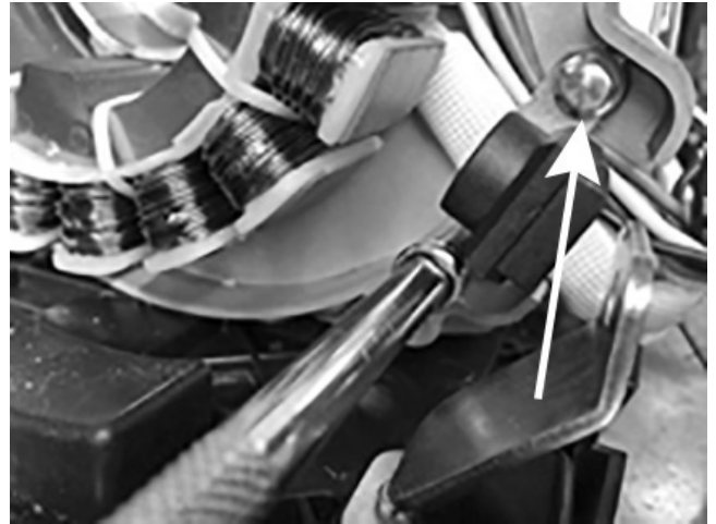
Figure 1-92. Adjustment Mounting Screws
