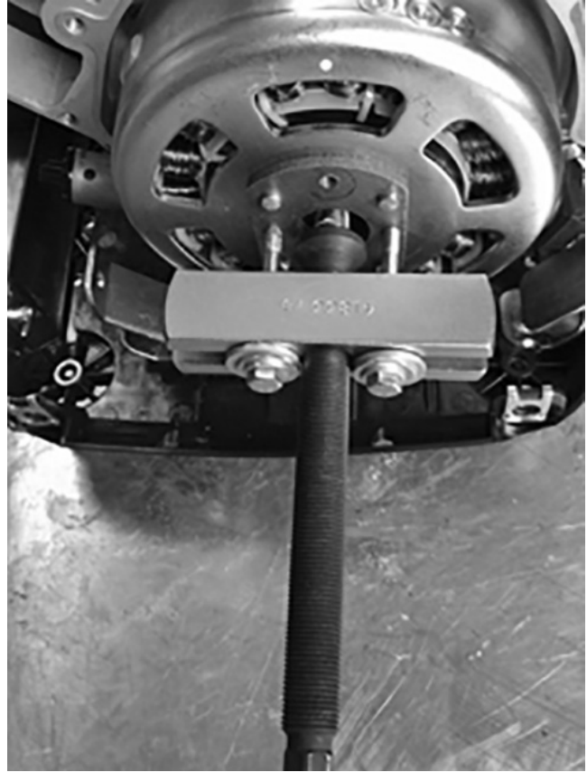
Figure 1-96. Remove Rotor with Puller
