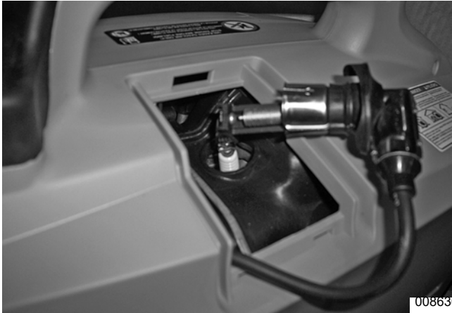
Figure 1-34. Ground Spark Tester
