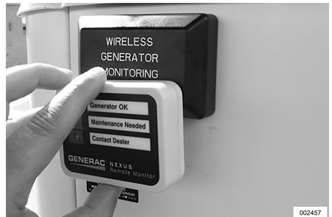
Figure 1-2. Place the Display Unit Against the Generator Transceiver
