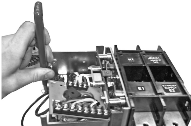
Figure 5. Ratcheting the Contactor
