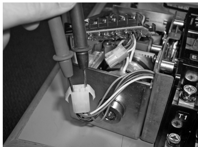
Figure 4. Measuring Resistance at Female Connector
