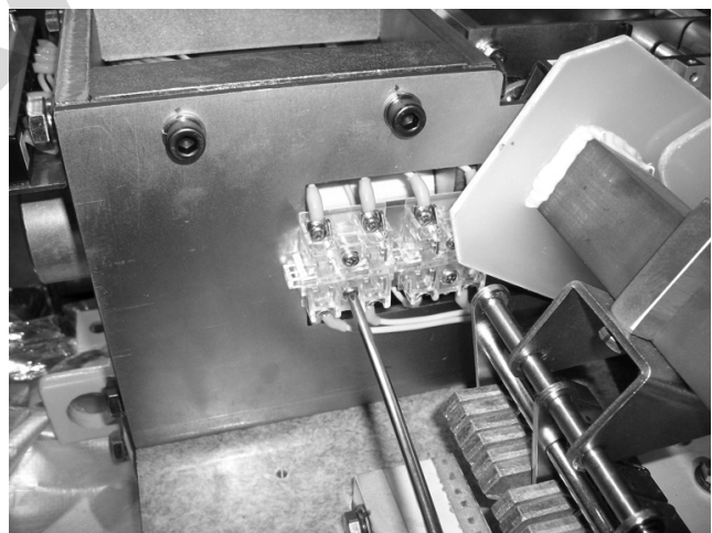
Figure 5. Replacing Limit Switches
