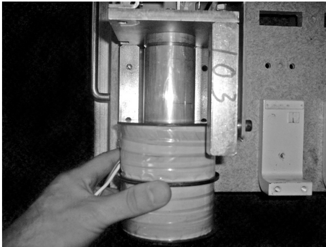
Figure 22. Slide Coil Off Plunger
