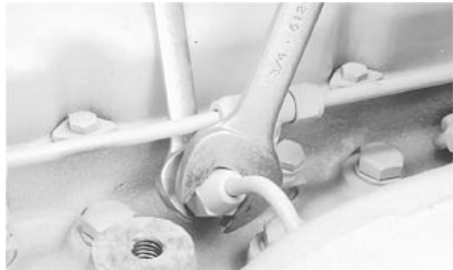
Bleeding Fuel System at Injection Nozzle
