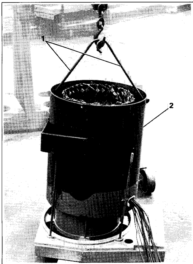
1. Lifting Hooks 2. Stator Figure 4-31. Stator Removal
