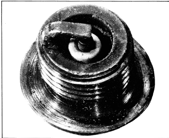
Normal: A plug taken from an engine operating under good conditions will have light tan or gray colored deposits. If the center electrode is not rounded off, a plug in this condition could be re-gapped and reused.
