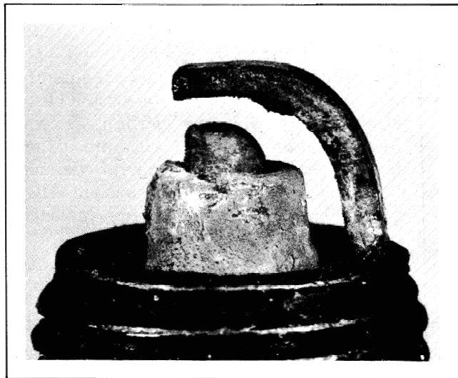
Worn: On a plug which has been in service too long, the center electrode will be rounded off and the gap will be eroded .010" or more than the correct setting. Replace worn plugs as they will require excessive voltage to fire properly. Always replace plugs in pairs.
