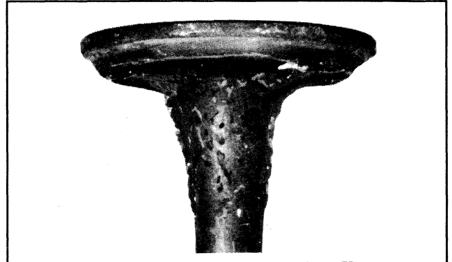
Gum: Gum deposits usually result from using stale gasoline. This condition is often noted in applications where fuel is not drained out of tank during the off season. Gum is a prevalent cause of valve sticking. The cure is to ream the valve guides and clean or replace the valves, depending on their condition.
