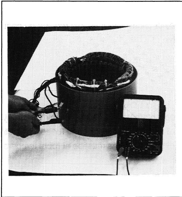
Figure 7-4. Testing Stator Windings
