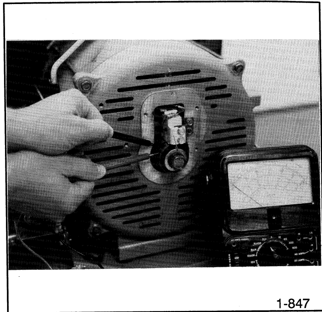
Figure 7-6. Rotor Resistance Check
