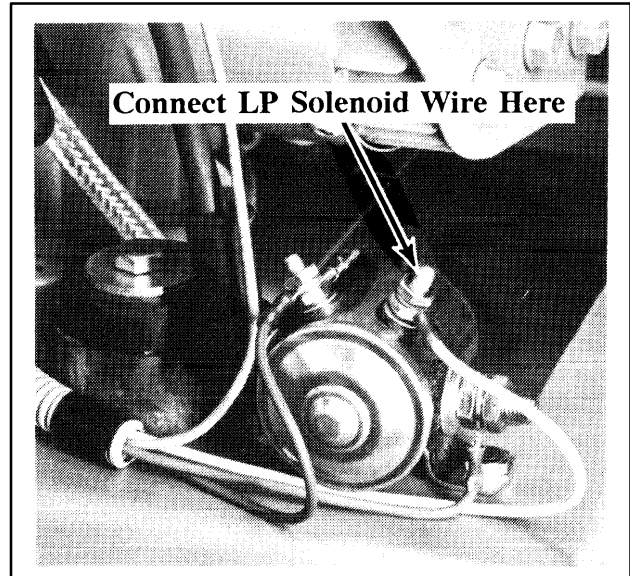
Figure 2. LP Fuel Solenoid Connection (if Equipped)
