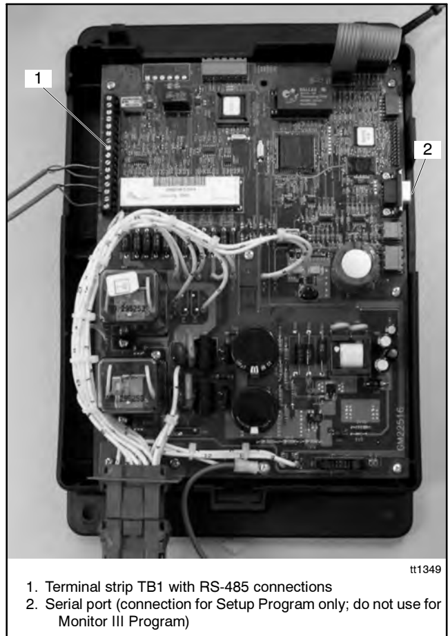
Figure 7-1 1000 ATS Controller (cover removed)
