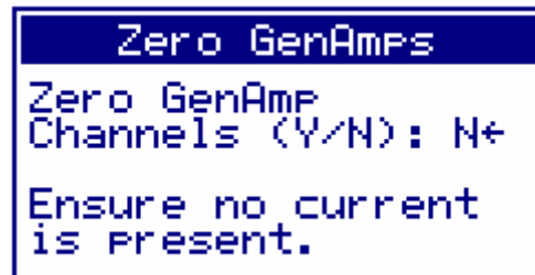
Figure 28 - Generator Current Zero Screen
