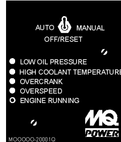
Figure 47. MPEC Engine Running Status LED
