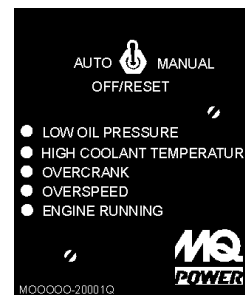
Figure 61. MPEC Engine Running Status LED (OFF)
