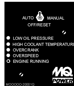
Figure 37. MPEC Engine Running Status LED
