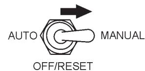
Figure 41. MPEC Control Switch (Manual Position)
