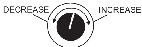
Figure 10. Voltage Regulator Control Knob
