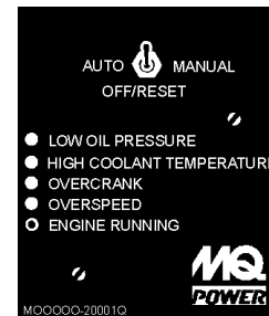
Figure 43. MPEC Engine Running Status LED
