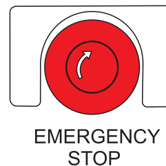
Figure 59. Emergency Stop Button
