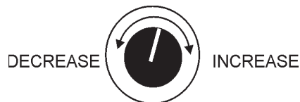
Figure 25. Voltage Regulator Knob (208V)
