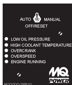
Figure 44. Engine Running LED (ON)
