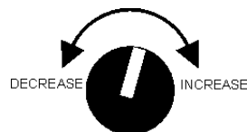
FIGURE 30. Voltage Regulator Knob located on the control panel
