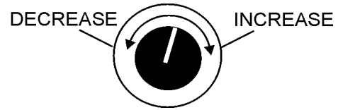
Figure 11. Voltage Regulator Control Knob
