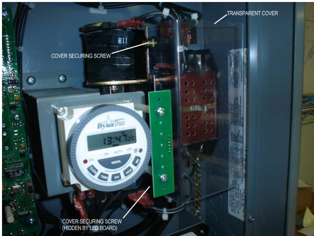
Figure 4. TRANSPARENT COVER SECURING SCREWS
