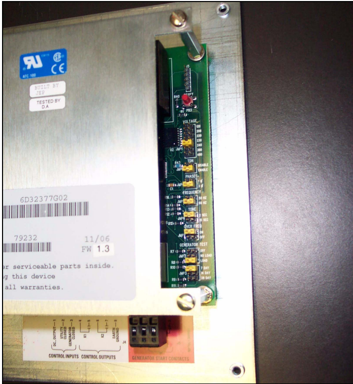
Figure 5. Jumpers on ATC-100.
