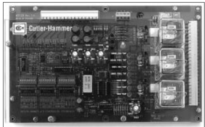
Figure 3-4 Microprocessor-based Logic Control Panel
