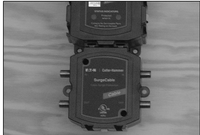
Figure 92. SurgeCable Mounted to the TVSS.
