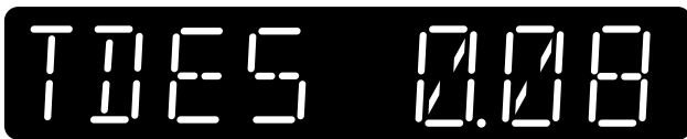
Figure 5. Typical Time Delay Normal to Emergency Time Display Upon Normal Source Loss
