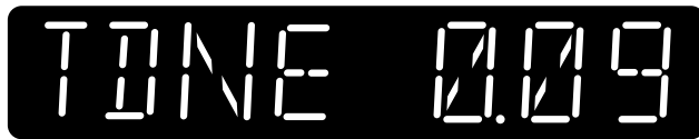
Figure 3-2 Typical Time Delay Normal to Emergency Time Display Upon Normal Source Loss
